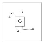
VC4V Pilot operated check valves works as a normal check valve for flow from port A to port B. Flow from port B to port A is blocked.
